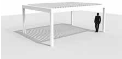
Stand-alone: the Camargue Line frame is supported by 4 vertical columns
