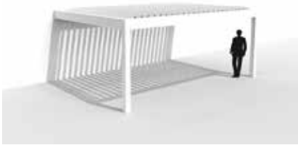
Façade mounting: the frame is placed with one or two sides against a supporting structure or structure behind it. Vertical columns support the other part. The blades can be placed parallel or perpendicular to the structure behind.
