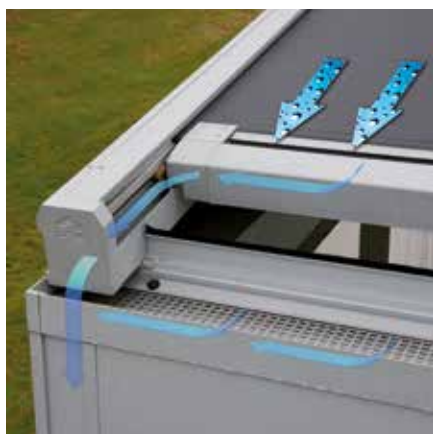
The Lagune can process a precipitation flow rate that corresponds to a rain shower with an intensity of 180 mm/h that lasts max. 2 minutes. This type of rain shower occurs approx. every 15 years. (Cf. Belgian rain statistics: standard NBN B 52-011)
